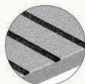
GROOVE WITH EPOXY FILLING
