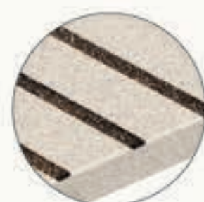
GROOVE WITH EPOXY FILLING
